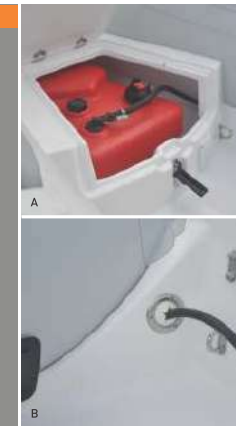
PICTURE A BOW LOCKER / SEAT TO FIT A PORTABLE FUEL TANK (9 TO 14) PICTURE B HIDDEN CHANNEL FOR FUEL LINE WITH SS STARBURST
